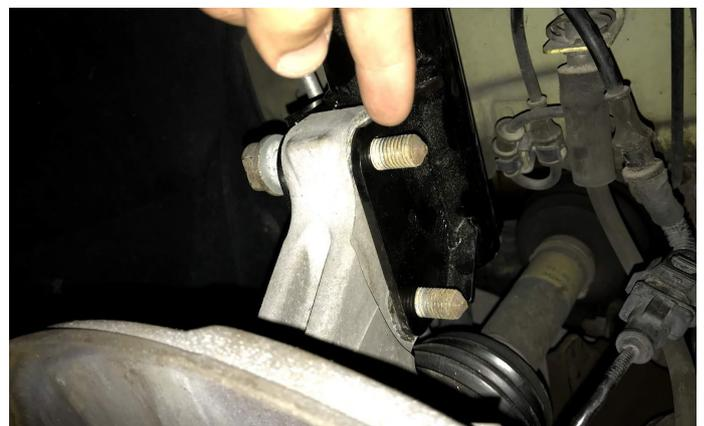
After this grab your new brake hose/wheel speed sensor wiring bracket and the paint marker. You will have to take this and line it up then notch it out to fit in the right area of the Maptun XT Series strut flush.
