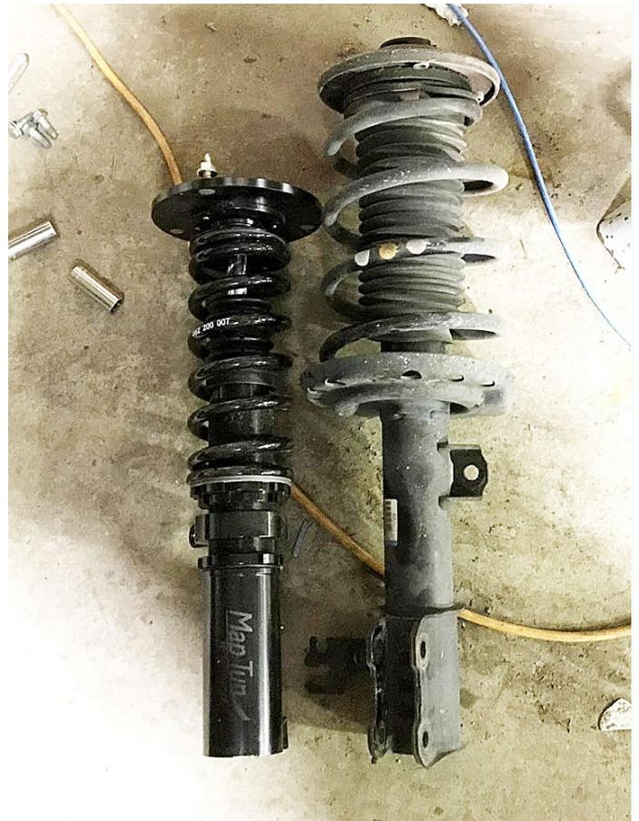
Before installation on the car, the spring must be adjusted to a default setting. Unscrew the lower spring seat (pos. A) so that the spring just makes contact with the upper and lower spring seats. After this, the lower spring seat is screwed up 5mm to get the correct pretension on the spring.
