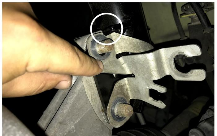
After fitting the notched out bracket tighten the nuts down and then add in the wheel speed sensor wiring then the brake hose with the clips removed from the factory strut.
