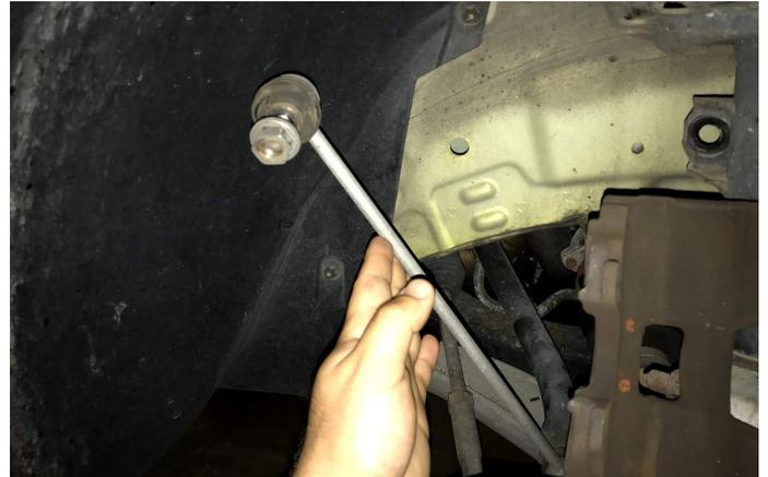
Next remove the brake line hold down and the wheel speed sensor wiring. You can use an angle pliers on all of this including the plastic hold down for the wheel speed sensor. Gently pull that off since it will be reused.
