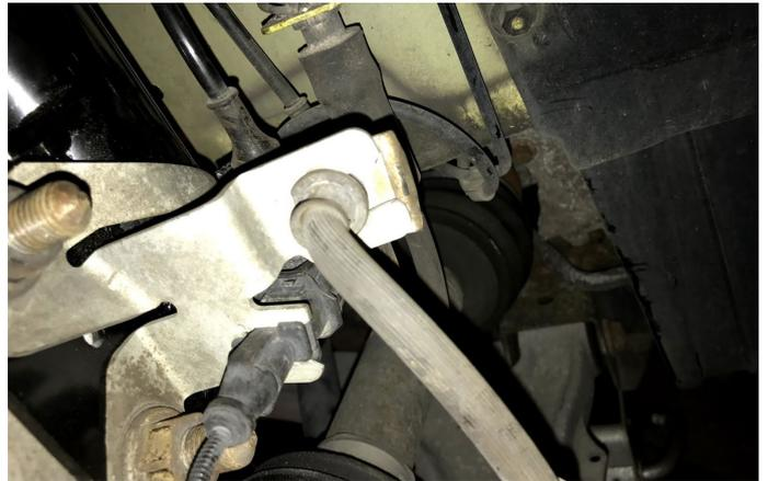
Once the brake hose and speed sensor wiring are back in place take the sway bar end link and line it up with the mount. Take the link and tighten it down then snug the set screw up. The set screw does not have to be cranked down, it just needs to be snugged up as to not cause damage to the threads.
