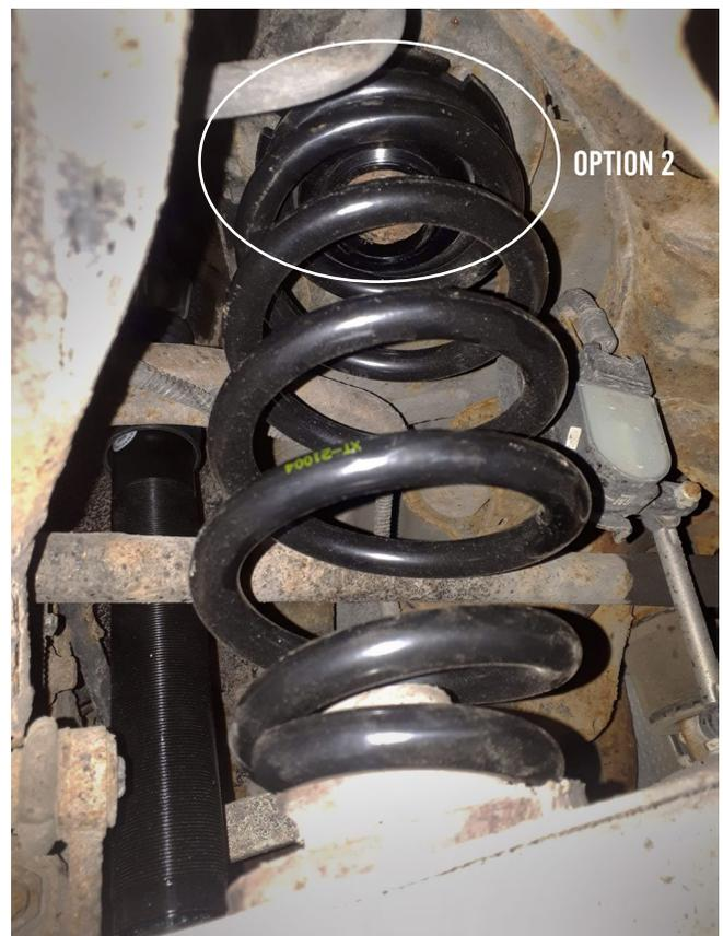
Choose one of the options and install the spring. Use the same option for both sides. Slowly raise the control arm with the jack so it meets the body (but does not lift the car off the stands). Reinstall the lower control arm bolt.
