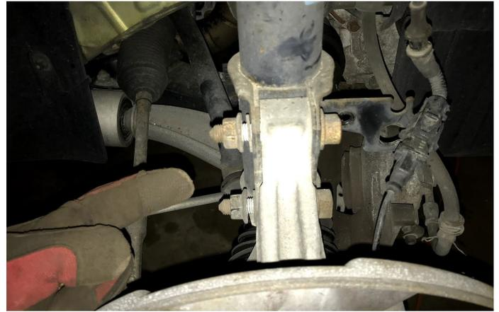
At this point you can remove the 3 bolts from the top and remove the strut.
