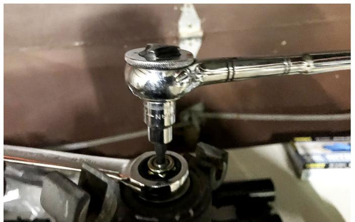
Once this is complete you're ready to reinstall the rear shock. Take the rear shock and cut the zip tie on the bottom. DO NOT LOSE, DAMAGE OR MISPLACE the other half of the bushing that comes out - its a two part bushing and must be installed that way. First attach the mount to the body and tighten down - then reinstall the bottom of the shock to the lower control arm.
